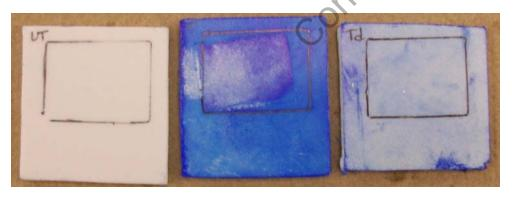
Left to Right: Untreated, Treated, Treated rubbed and rinsed. Samples BPB direct stained. Black lines indicate where JIS Z2801 inoculum was placed. Blue stain indicates presence of antimicrobial.
